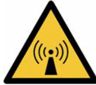
W005 Warning; Non-ionizing radiation
