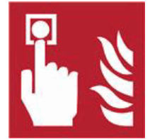
F005 Fire alarm call point
