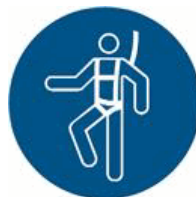
M018 Wear a safety harness
