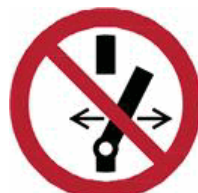
P031 Do not alter the state of the switch
