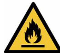
W021 Warning; Flammable material
