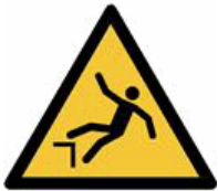
W008 Warning; Drop (fall)
