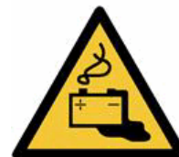
W026 Warning; Battery charging
