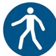
M024 Use this walkway
