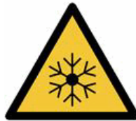
W010 Warning; Low temperature-freezing
