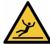
W011 Warning; Slipper surface
