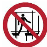
P025 Do not use this incomplete scaffold
