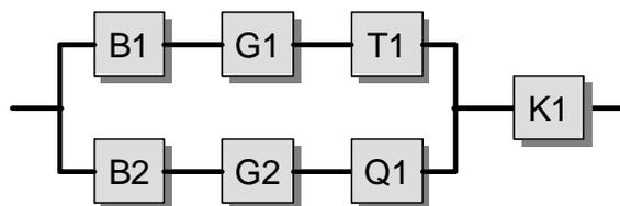
cation software. The actual rotational speed value of the inching speed on the inputs I3.0 and I3.1 of K1 is monitored by two separate tachogenerators G1 and G2. Each channel of the PLC performs the desired/actual speed comparison independently. Should the speed not be reduced successfully to the limited value by means of T1, K1 can initiate a halt by blocking of the start/stop signal and pulse blocking on the inverter. The power supply to T1 can also be interrupted by a mains contactor Q1.
