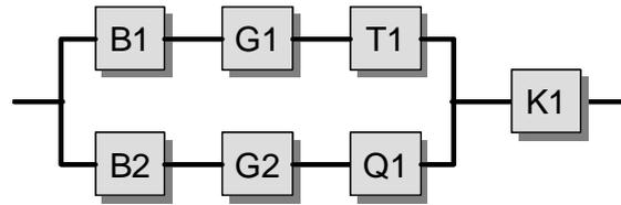
process; the mains contactor Q1 is monitored directly by the PLC. These values produce a  $DC_{avg}$  of 99% (“high”).
