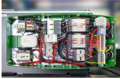
Wire rope hoist, control box opened, full control system visible (19)
