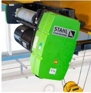
Wire rope hoist, control system located inside the green control box (18)
